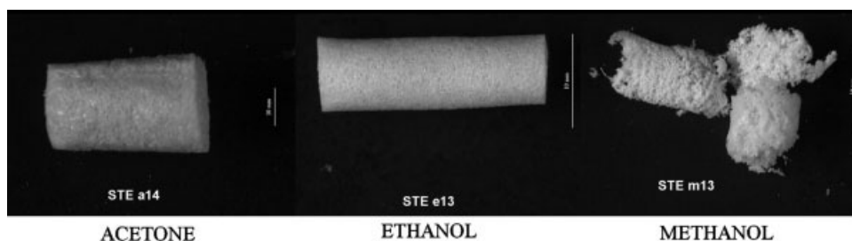
Figure 2 DBC scaffold samples produced by using different solvents.
